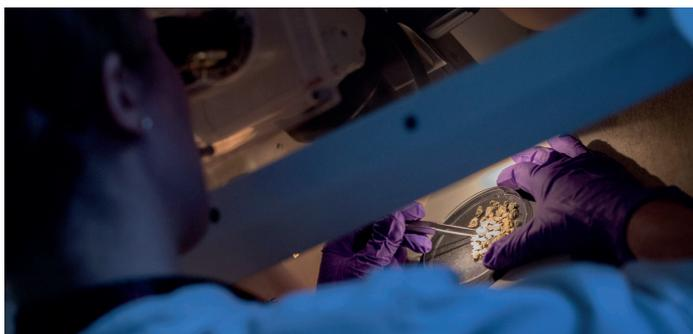
For bulk samples where no fibres have been observed using the stereo microscope or no asbestos fibres have been identified by PLM, at least two microscope slide preparations of randomly selected representative materials are made for examination by PLM.
