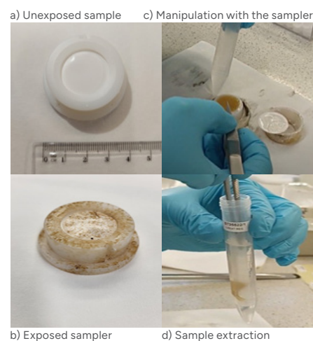
Figure 2: The LSNW-AP sampler for PFAS water sampling and its laboratory extraction.
